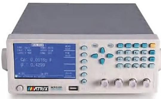
MCR5000 series is a multifunctional LCR precision meter used for testing various electronic components. Adopt 4.3-inch TFT LCD display, simple display, elegant layout. It is a high speed, wide band, 5 bit test resolution impedance measuring instrument with 40hz-200khz multiple frequency points and 0.1% accuracy, which can meet the requirements of component parameter detection in various occasions. Is a high - quality cost-effective tester
