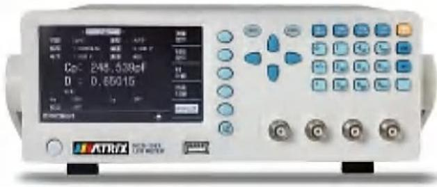
LCR 6000A series high-precision digital bridge is a multi-function component parameter tester for detecting various electronic components. Tell, stable, 12Hz-600kHz continuous frequency point and 0.05% accuracy, can meet the requirements of production line quality control, purchase inspection and laboratory measurement, etc.
